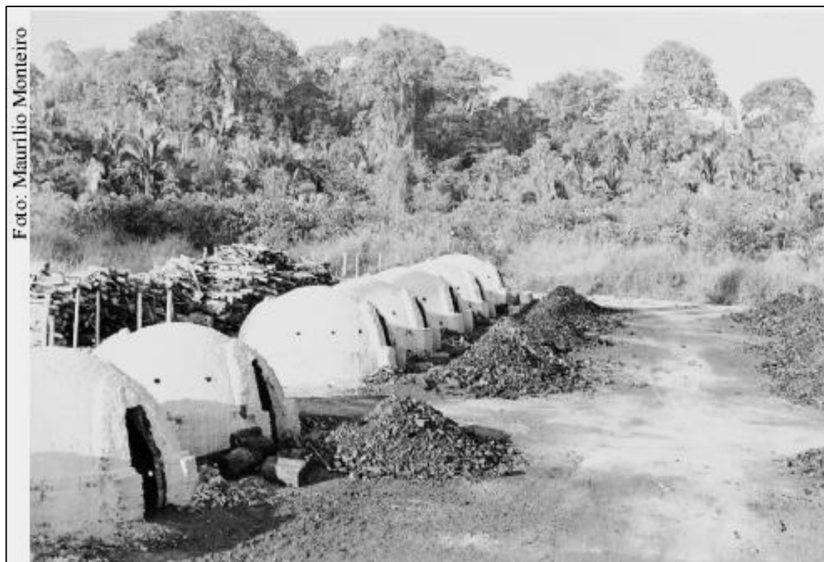
Figure 9. Rabo-quente kilns for charcoal production
